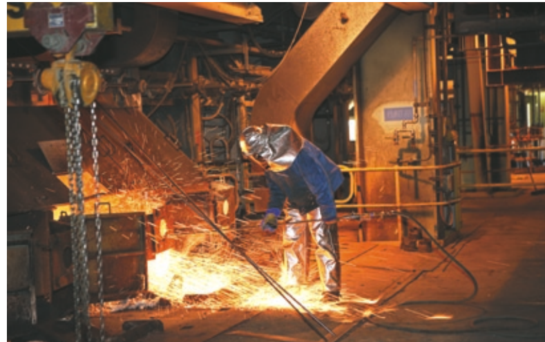
Plate 22.2 Engineered fume extraction and personal protective equipment used by a smelter tapper
