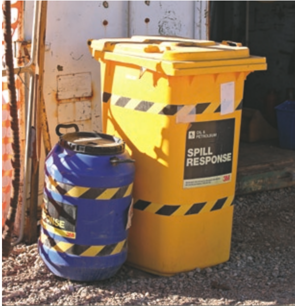
Plate 22.8 Spill response equipment used at existing operation
