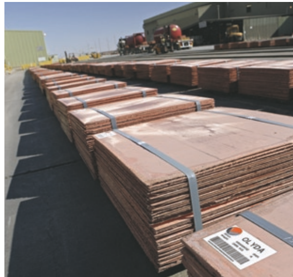
Plate 3.1 Copper is transported from Olympic Dam as copper cathodes
