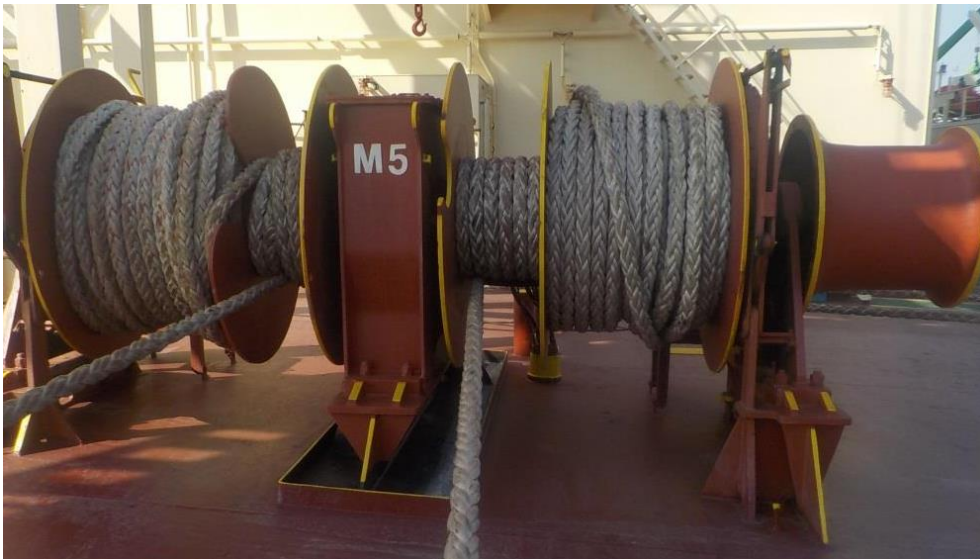
Photo 2: Split drum design mooring winch
